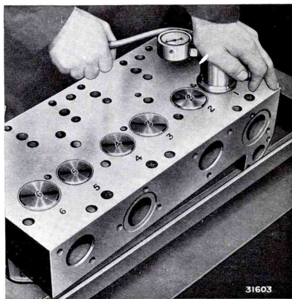
FIG. 25. TESTING GAS-TIGHTNESS OF VALVE ON ITS SEAT
