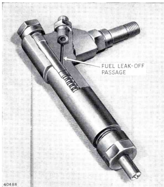
FIG. 61. PART SECTIONED VIEW OF INJECTOR UNIT
