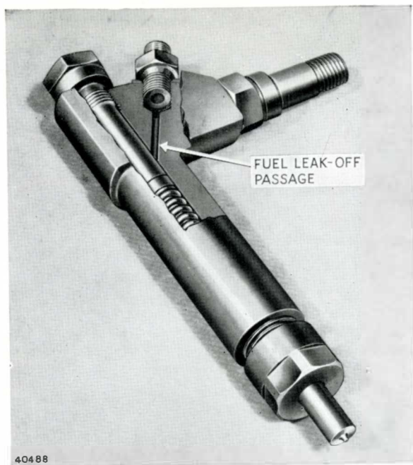
FIG. 60. PART SECTIONED VIEW OF INJECTOR UNIT
