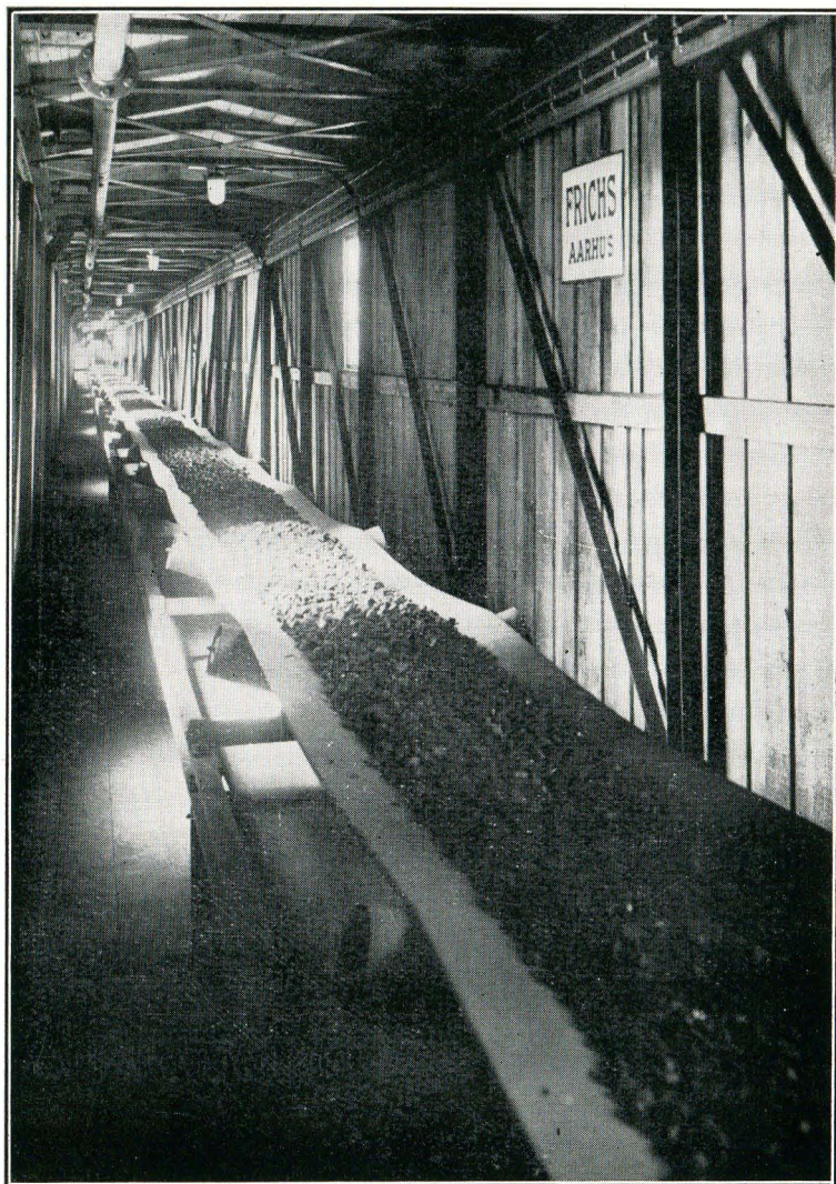
TRANSPORTBAAND FOR KUL - KAPACITET: 50 TONS PR. TIME BELT CONVEYOR FOR COAL - CAPACITY: 50 TONS PER HOUR
